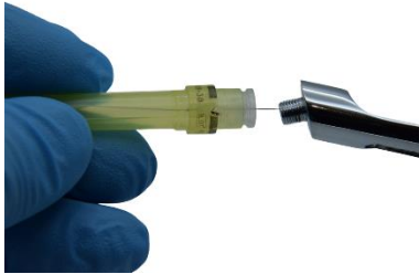
Figure 1: Insert the Needle to the top edge of the opening, placing the needle in straight.
